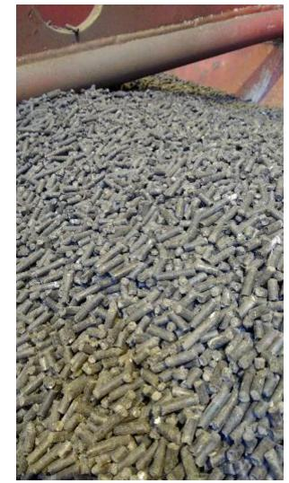
Shredder fraction: PCBs shredded (approx. 9% Cu)
