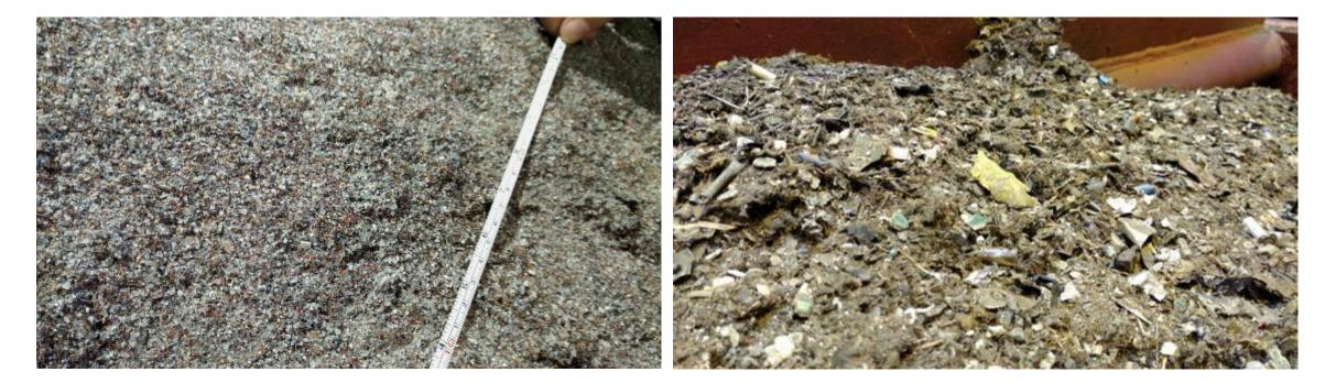
Shredder fraction: Cu wet (approx. 15% Cu) Shredder fraction: shredder fines/ light shredder fraction/ fluff (approx. 10% Cu)
