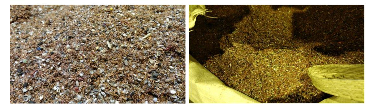
Shredder fraction: Cu coarse (approx. 70% Cu) Shredder fraction: Cu fine (approx. 65% Cu)
