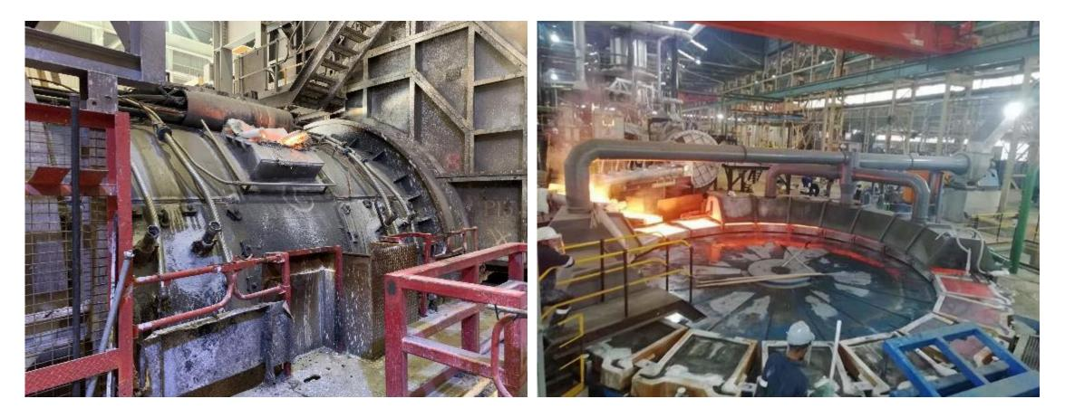
Anode furnace for pyrometallurgical refining
