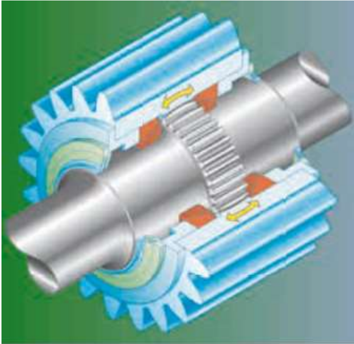
Drive pinion of the COMBIFLEX® drive: the self-aligning drive pinions compensate wobbling of the girth gear.
